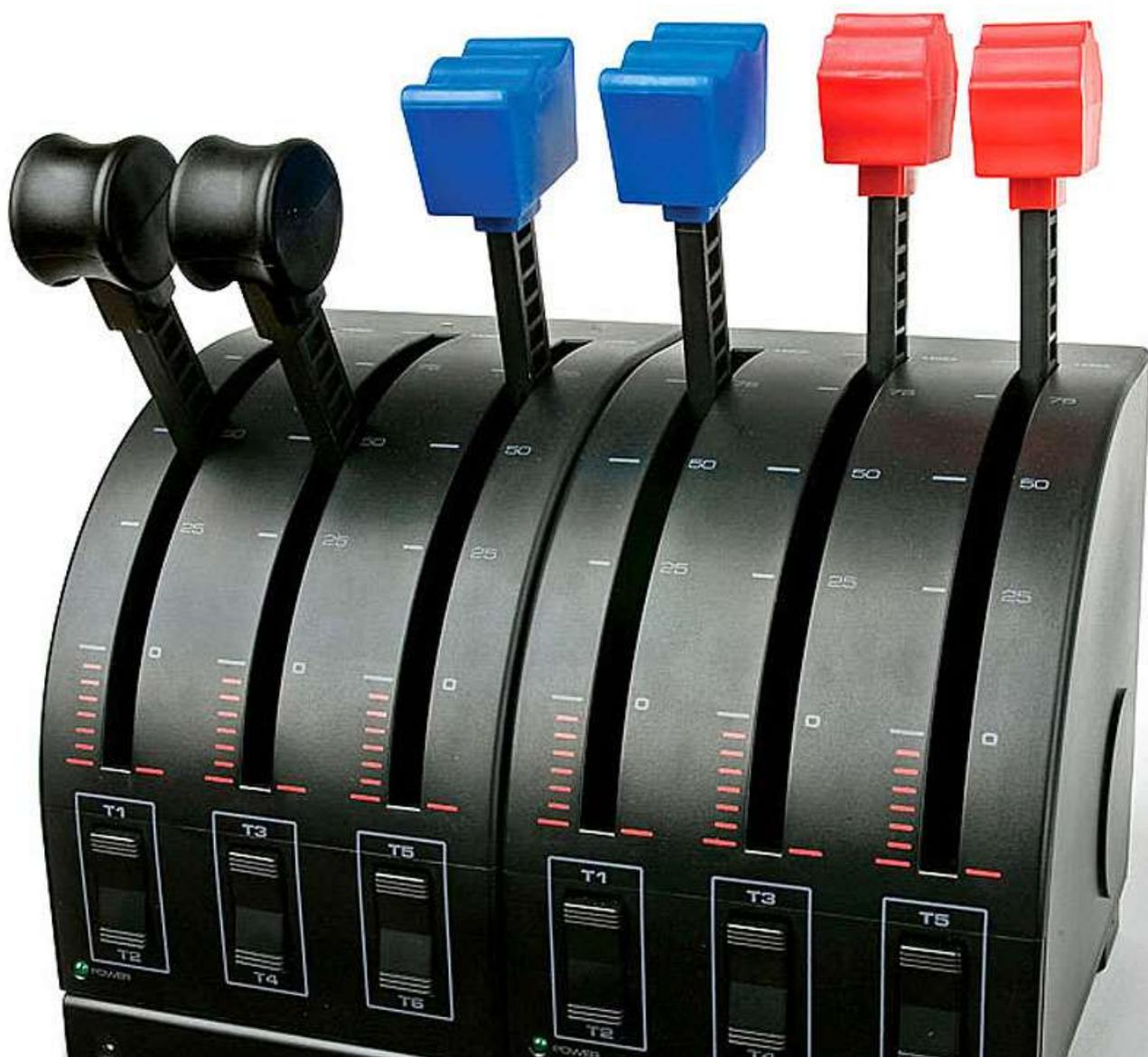
Each quadrant comes with a clamp that the user can screw to either the bottom or the back of the unit, allowing to install the quadrant on the border of a table. This is good for permanent or occasional use, but is less than convenient if you need to install/uninstall the quadrant(s) quickly, for instance if you use the computer for other activities yet you wish every day to do some flightsimimming.
