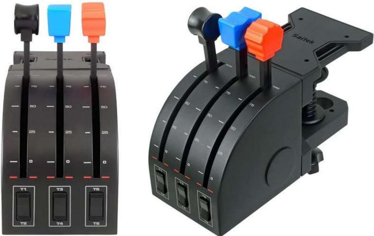
**Installing the hardware.** Each quadrant comes with knobs inserted for the default one-engine setup: from left to right there is a black knob for throttle, a blue knob for propeller RPM and a red knob for mixture or condition. Quite obviously, for a twin quadrant you should exchange the handles so that you have, from left to right, two throttles, two propellers RPM and two mixtures or conditions.
